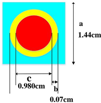
**Figure 3.** Configuration of the pin-cell benchmark [9]
