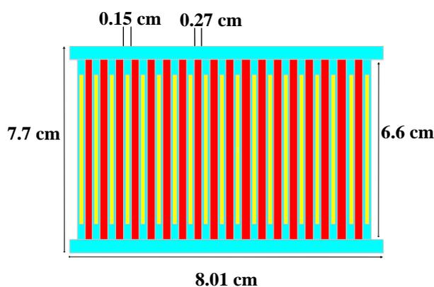
Figure 4. 2D TRR fuel box schematic [12]
