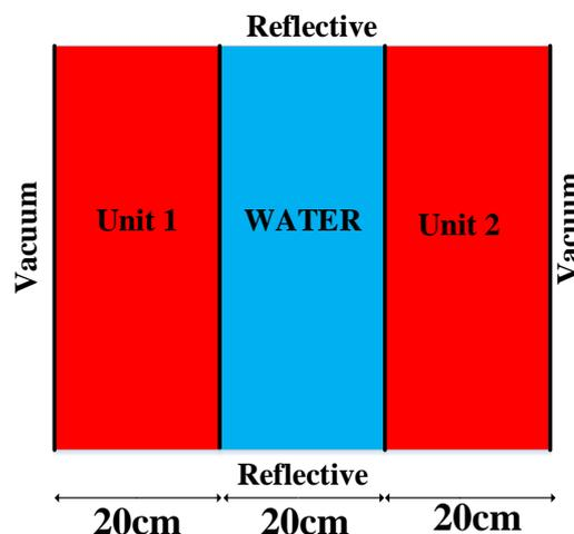
Figure 2. Geometry of slab benchmark problem[11]
