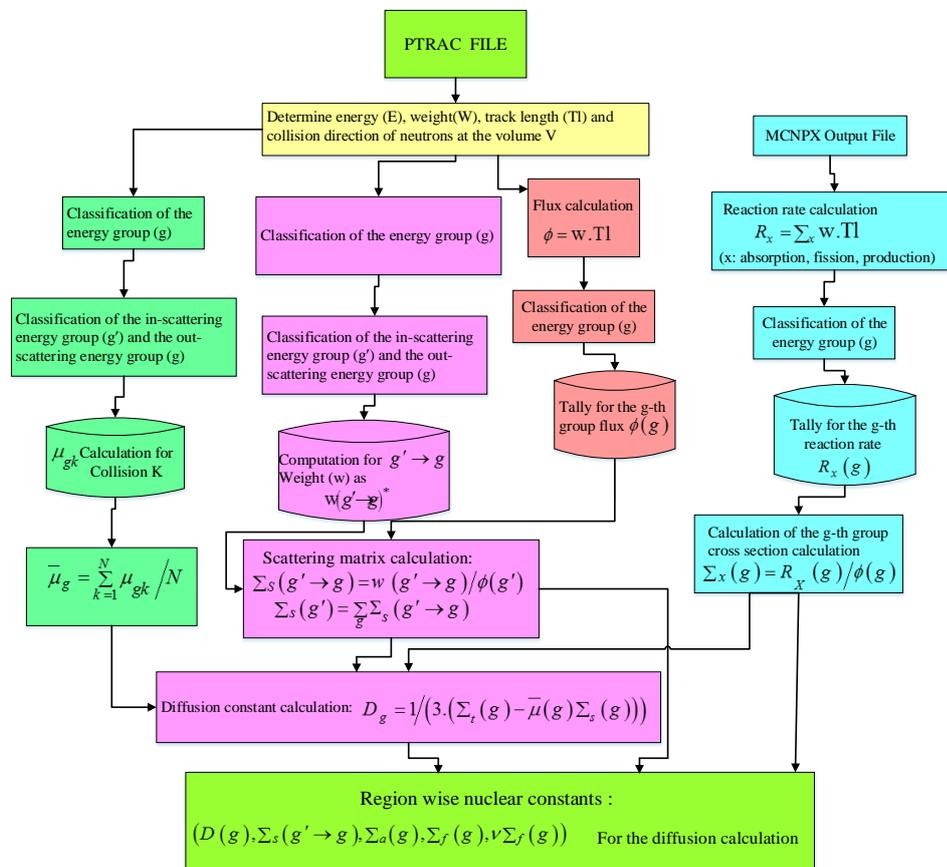
Figure 1. Block diagram of the methodology used in this study for multi-group constants generation.
