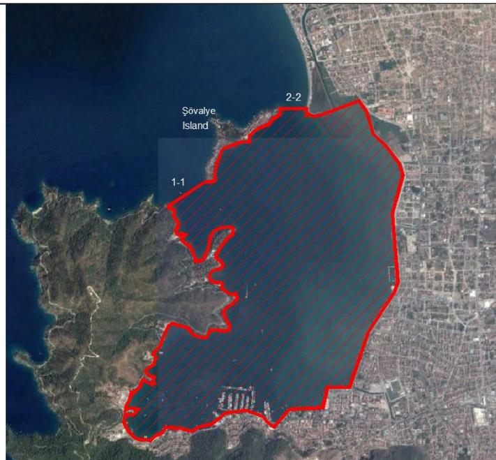
**Figure 3.** Computational cell utilized for the inner bay of Fethiye to simulate the mean water quality parameters. [20]
