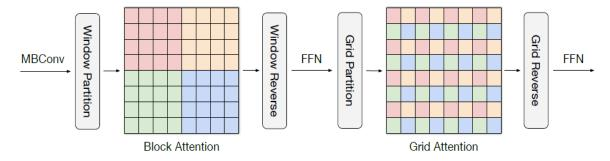
**Figure 2.** A Depiction of the Method for Calculating Self-attention using a Multi-axis Approach, with a Window/grid size of 4x4 (Tu et al., 2022).
