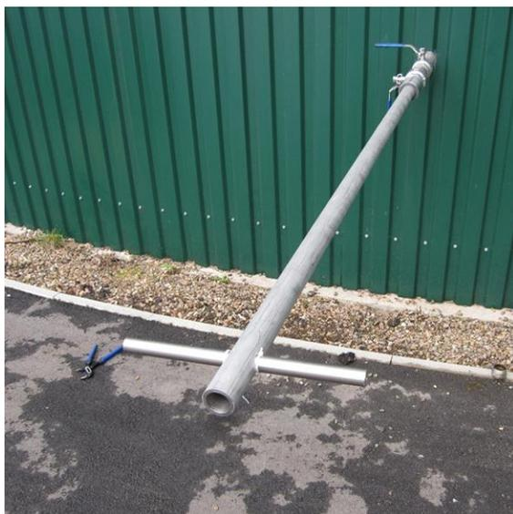
**Fig 2.** Measuring rod used for the velocity measurements
