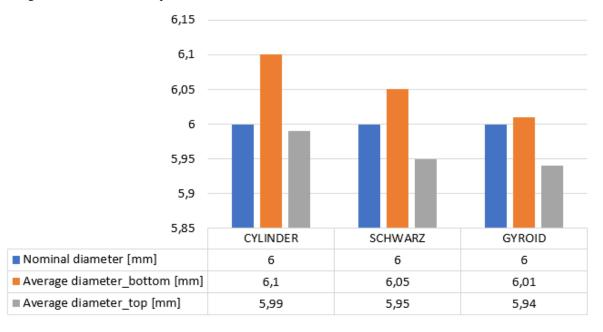
Figure 13. Average outer diameter measured from the lower surface, average outer diameter measured from the upper surface, nominal outer diameter dimensions of all models
