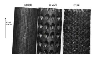
Figure 8. 3D printed TPMS based nerve guide conduits
