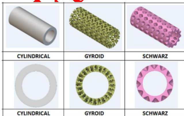
Figure 5. Perspective and top views of nerve guide conduits design models
