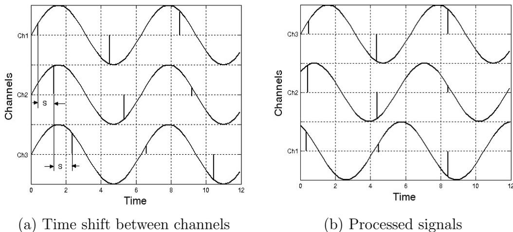
FIGURE 1. An illustration of a signal phase shift between adjacent channels.
