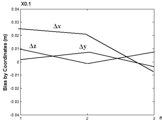
FIGURE 6. The error reduction in measurement of coordinates of a signal source in frequency domain.
