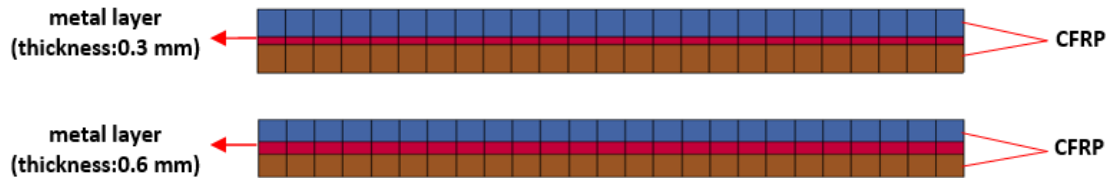
Figure 4. The side view of a FEM model of the hybrid composite laminates tensile test specimens.
