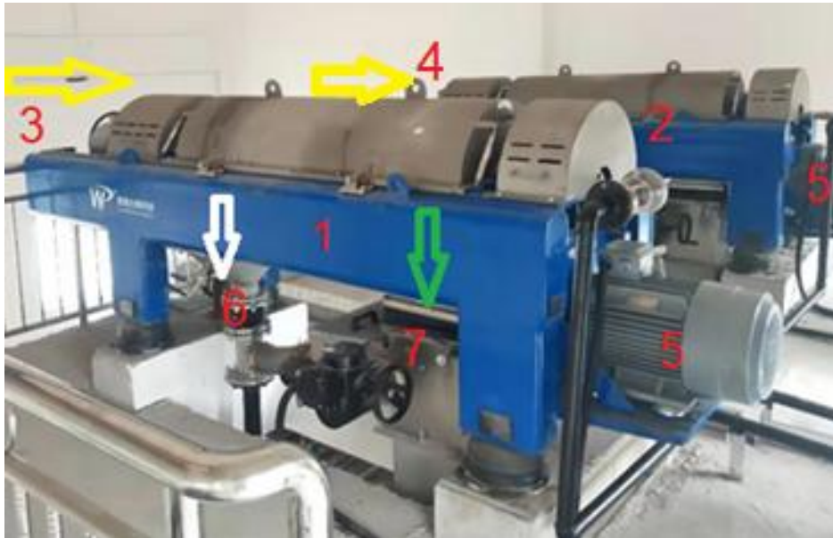
Figure 1. The decanter unit considered in this study 1&2 Decanter units (main and spare one), 3&4 Sludge feeding, 5 Decanter electric motor 6-Separated liquid output 7-Separated solid output
