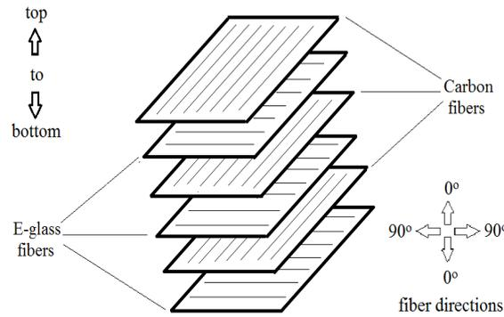
**Figure 1:** Design of hybrid composite without PA66.
