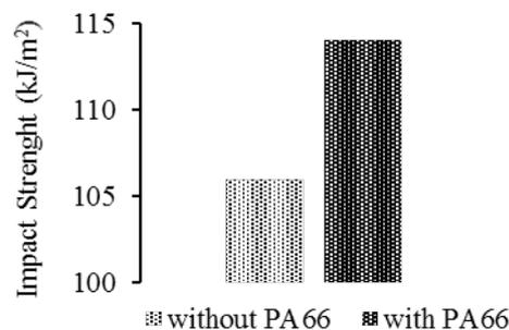
**Figure 3:** Impact strength of composites
