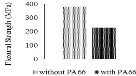
**Figure 4:** Flexural strength of composites.
