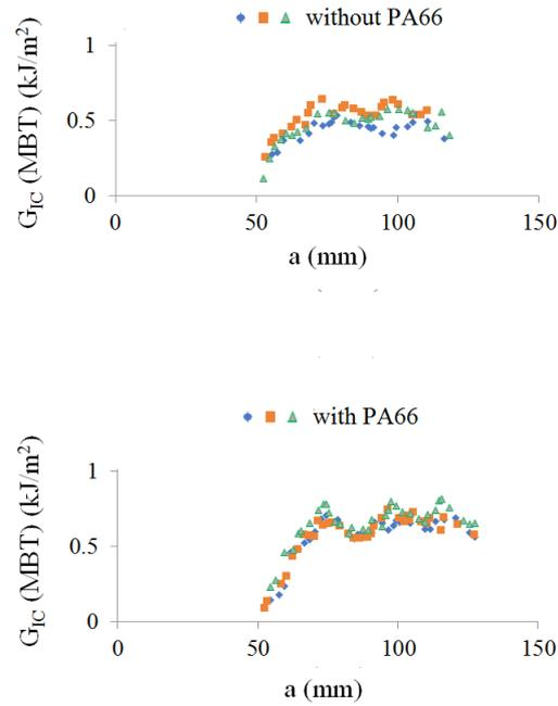
**Figure 5:** Mode-I interlaminar fracture toughness of composites.
