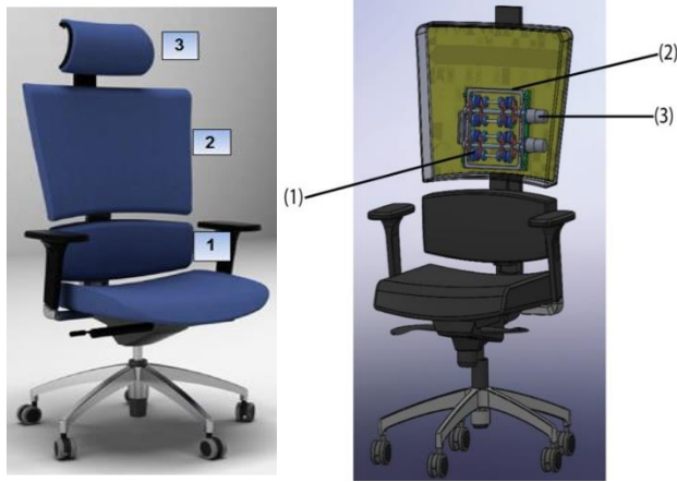
Figure 1. a. Office chair designed in the scope of San-Tez Project (1: Waist, 2: Back, 3: Neck) b. The office chair with a kneading massage mechanism (1: Massage wheels, 2: Mechanism body, 3: Electric motor) [5].
