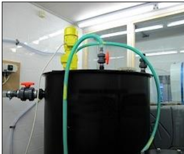
Photo 5. The bread digester for renewable energy (Biogas) in the Netherlands. Source: Enki Energy, by Stefan Blankenburg, 2016.
