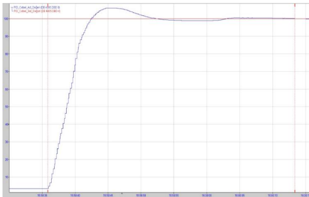
Figure 9. S7-300 PID (proportional-integral-derivative) graph ( K_p=5, K_i=2, K_d=1 )
