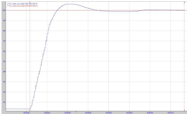
Figure 9. S7-300 PID (proportional-integral-derivative) graph ( K_p=5 , K_i=2 , K_d=1 )
