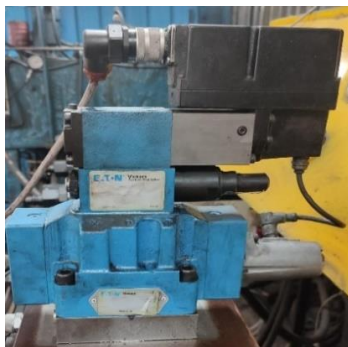
Figure. Hydraulic proportional valve and Experimental setup installed with S7-300 PLC
