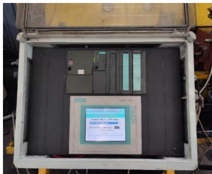
Figure. Hydraulic proportional valve and Experimental setup installed with S7-300 PLC
