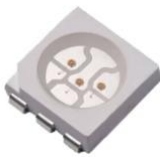
Figure 2. SMD 5050 RGB LED chip (left) and RGB LED module (right).
