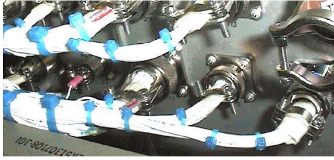
Figure 4. Proper practice of stress relief.
