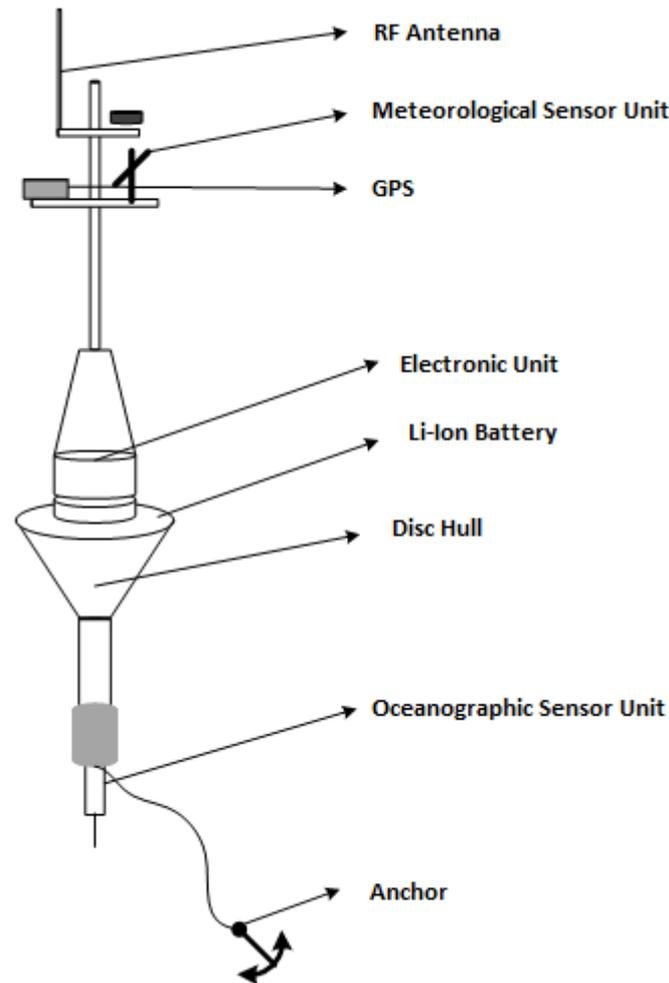
**Figure 2.** Concep variant-3 of the buoy design.
