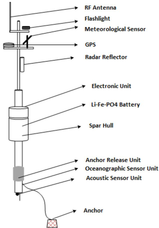
**Figure 1.** Concep variant-2 of the buoy design.
