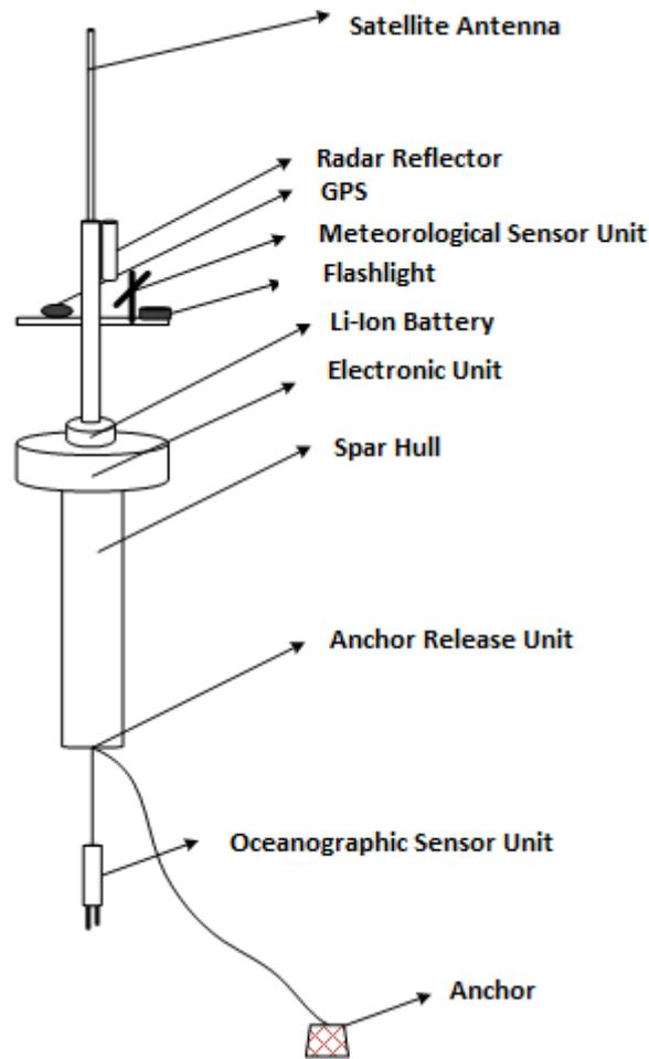
*Figure 3. Concep variant-5 of the buoy design.*
