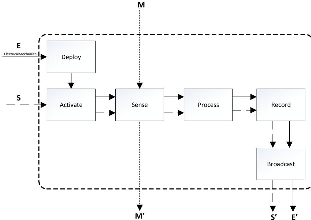
*Figure 1. A sample function structure of the marine surveillance buoy.*
