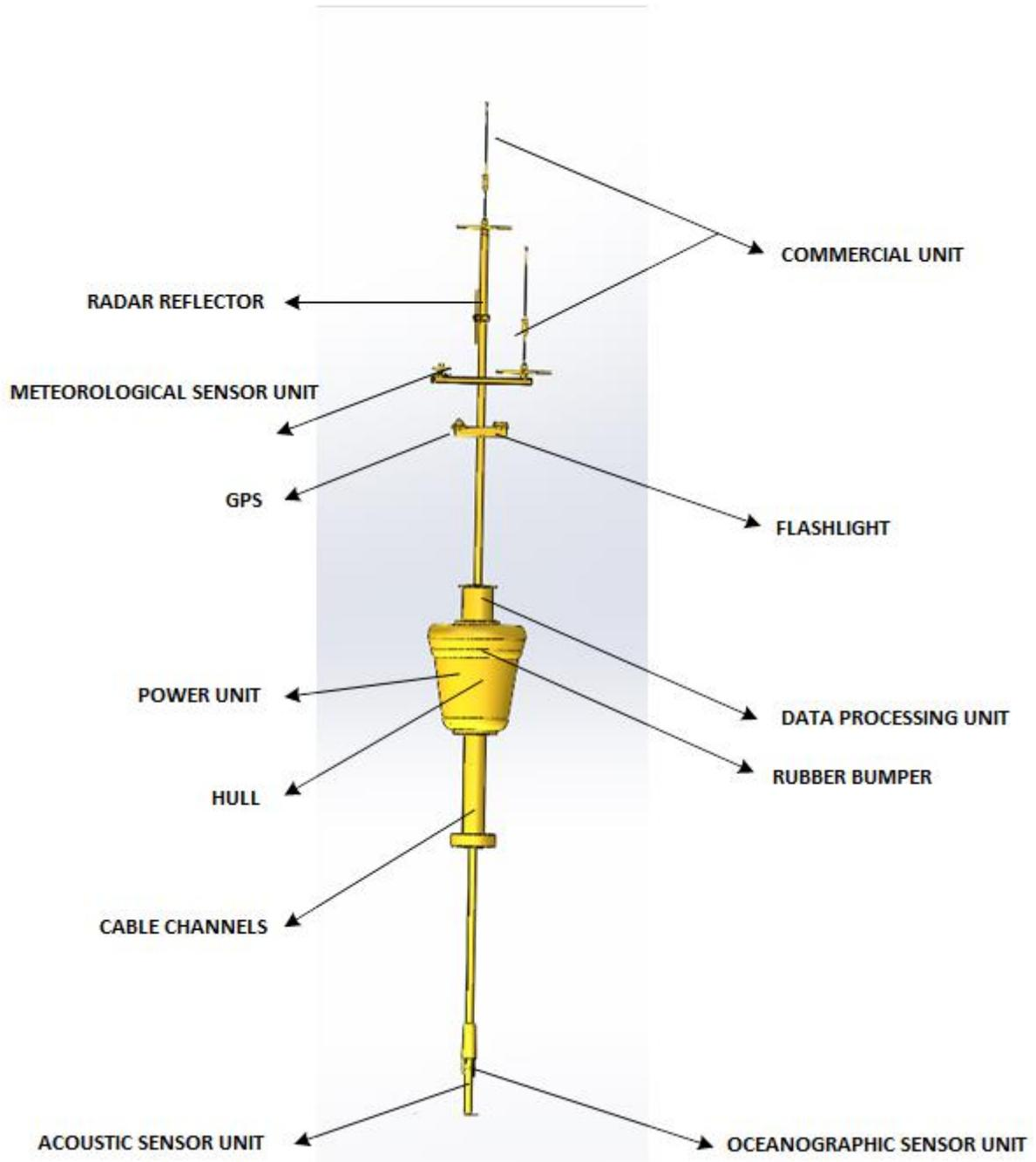
**Figure 6.** The chosen as the best design variants of buoy concepts.
