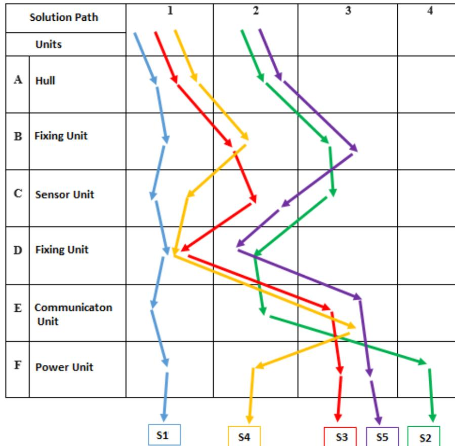
**Figure 3.** Concept variants of the buoy design (general designs).
