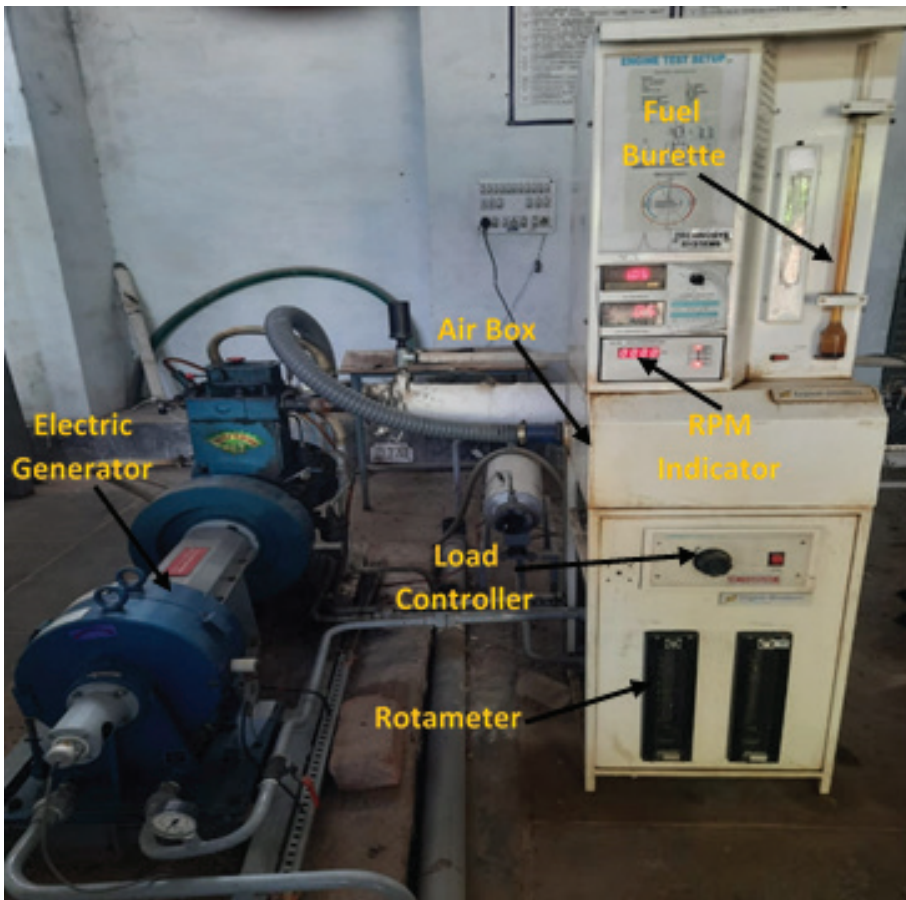
Figure 4. Diesel engine test rig with measuring device.
