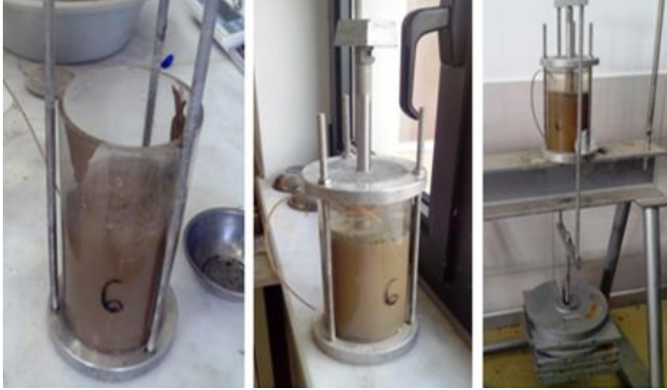
Figure 5. Soil consolidation phase
