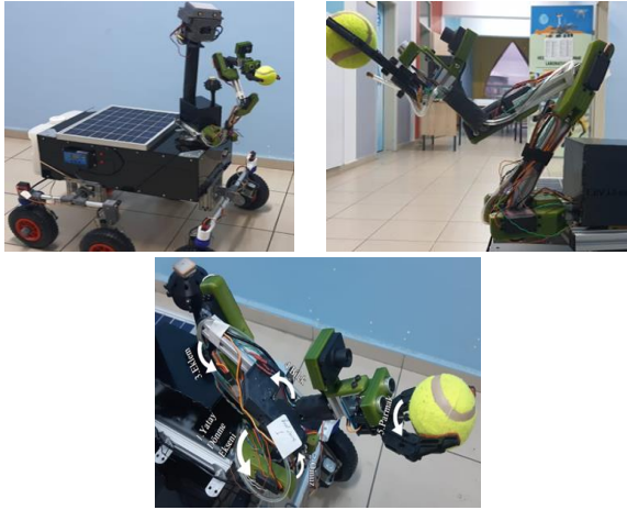
Figure 5. Images of the Designed Robot Arm. These images show the D.O.F. structure of the robot arm, the way it grips objects, the design structure of the arm, motors, camera and distance sensor.
