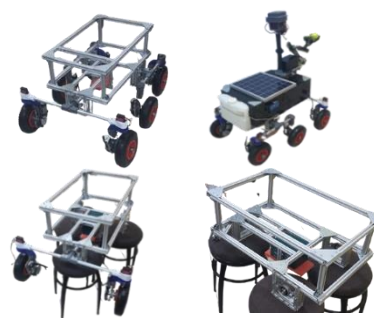
Figure 4. The body frame of the robot
