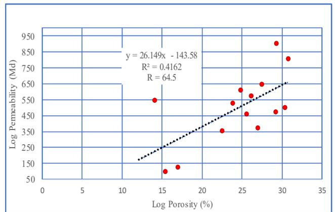
Fig. 6. The plot of log porosity against log permeability
