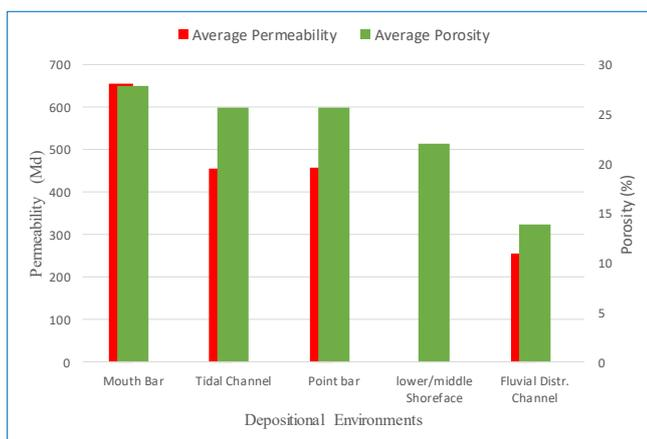
Fig. 5. The variations of Permeability and porosity values with the environments of deposition
