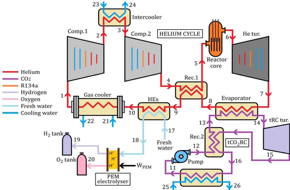
Figure 2. Schematic drawing of a GCMR integrated with the tRC cycle and H<sub>2</sub> production.
