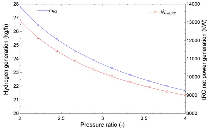
**Figure 12.** Impact of pressure ratio on  $H_2$  generation and tRC net power generation
