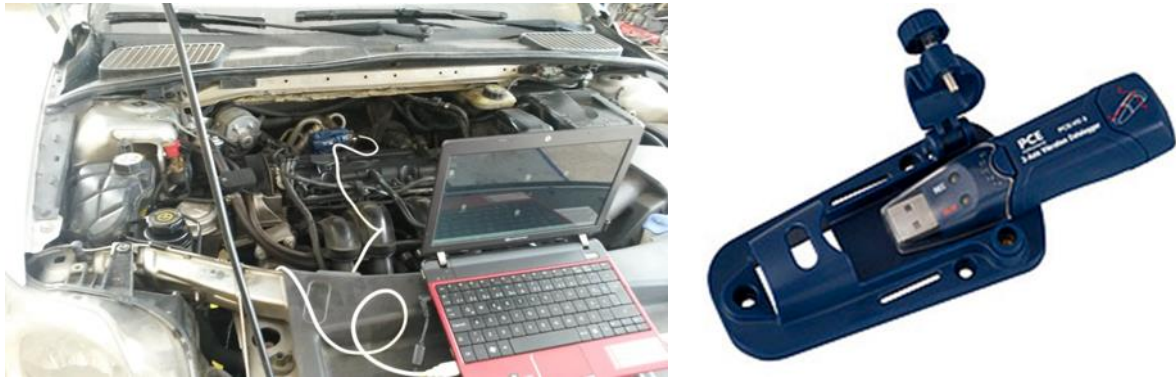
Fig. 1. The experiments equipment: the gasoline engine using LPG (a) and the accelerometer (b)
