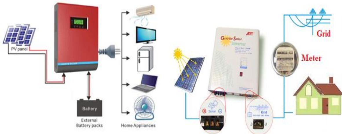
a) Off-grid inverter including charge controller
