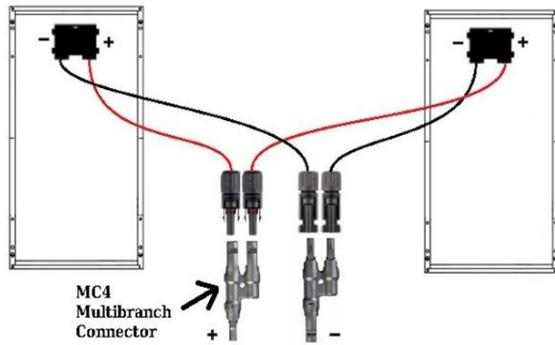
Fig. 9. Cable with connectors [26].
