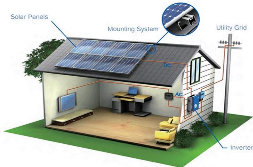
Fig. 5. On-grid residential solar PV system [17].
