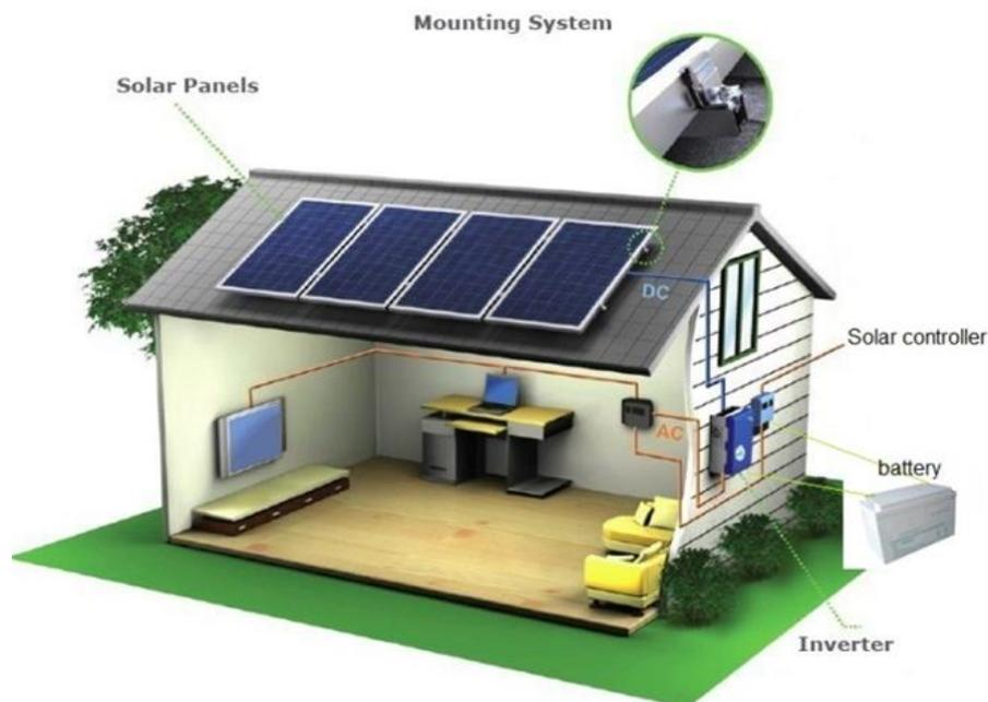
Fig. 4. Off-grid residential solar PV system [16].
