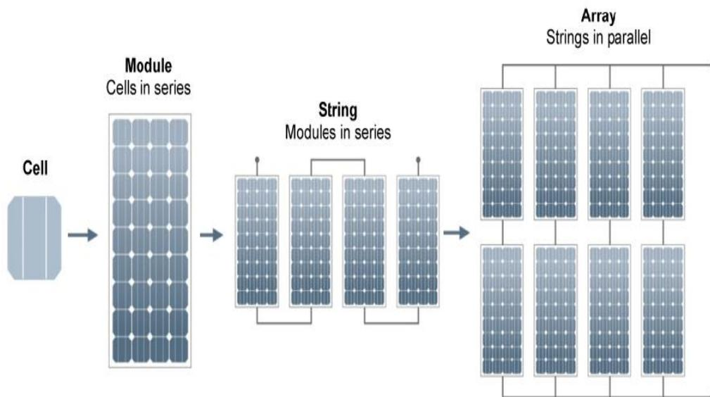
Fig. 6. From solar cell to solar array [19].
