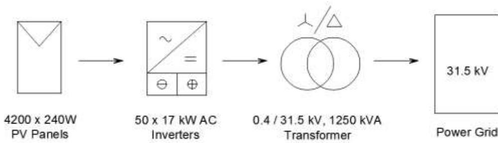
Figure 1. General structure of the solar power plant
