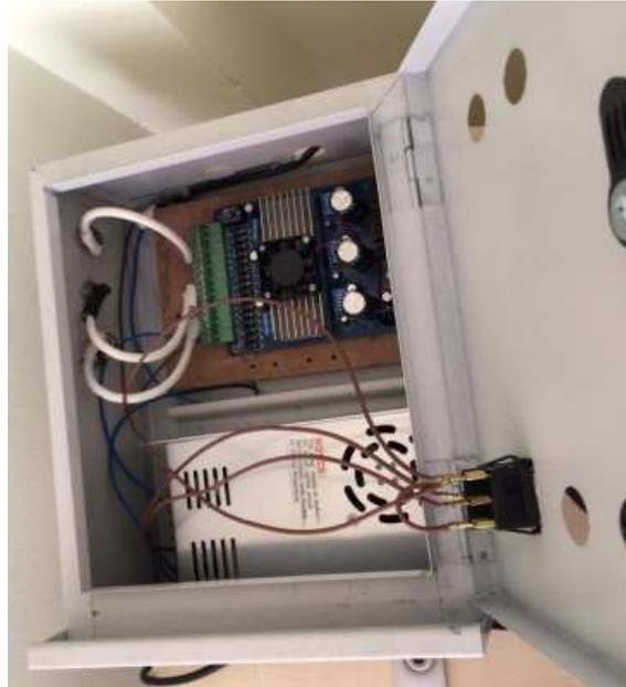
**Figure 9. Driver Card and Power Supply Panel**
