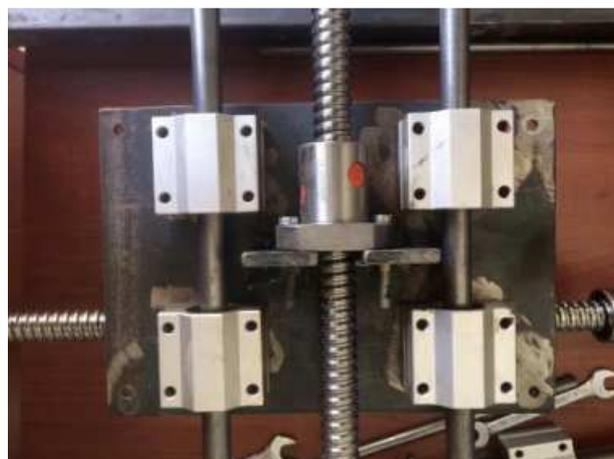
*Figure 8. Ball Screw Nut*
