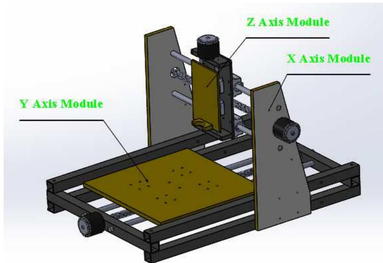
*Figure 3. Solid Model of a three-axis Mini CNC Machine*
