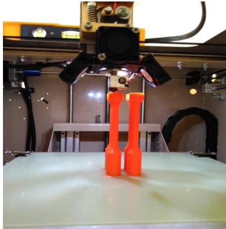
**Figure 4.** Printed standard tensile test samples
