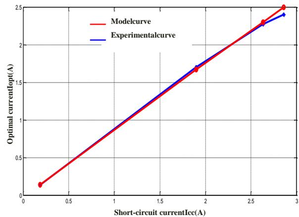
Fig. 9. Variation of the optimal current according to short-circuit current.
