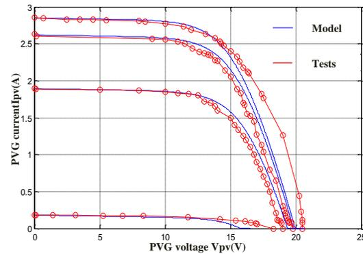
Fig. 8. Validation of our model using the curve previously obtained.
