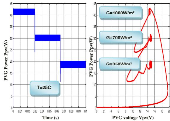
Fig. 12. Variation of the PVG power for a constant temperature and variable illuminations.
