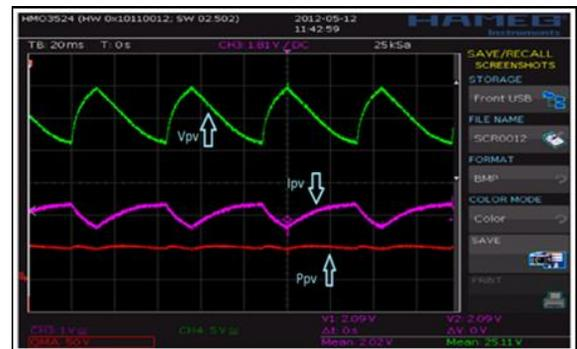
a. PVG current, voltage and power, with 3 batteries (12V, 150Ah).
