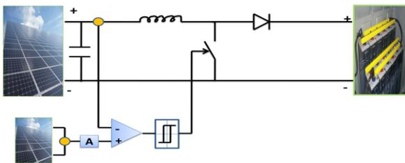
Fig. 10.Control circuit of the boost converter.
