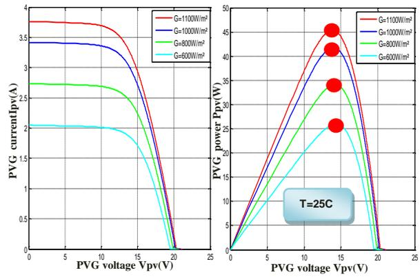
Fig. 4. PVG (current- voltage) and (power- voltage) characteristic for different solar illuminations.
