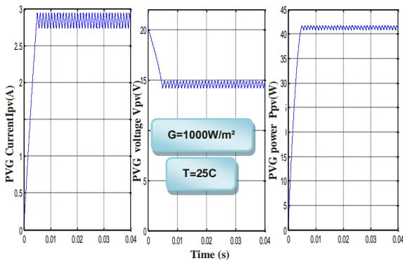
Fig. 11.Variation of the current, the voltage and PVG power for a constant illumination and temperature.
