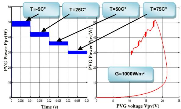
Fig. 13. Variation of the PVG power for a constant illumination and variable temperature.
