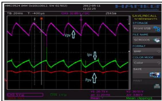
b. PVG current, voltage and power, with resistor load ( $R=30\Omega$ ).
