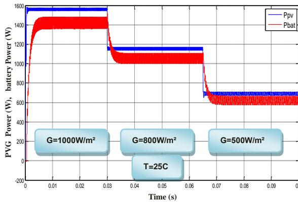
Fig. 16. Variation of the PVG and battery current for a constant temperature and variable illumination.
