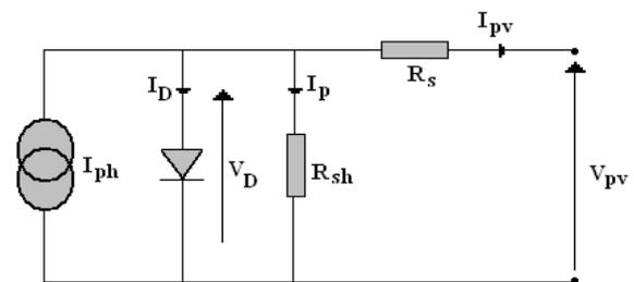
Fig.1.Simple model of the photovoltaic cells.
