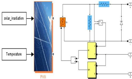
Fig. 2. Structure of the PVG Simulink model.
