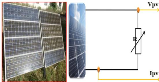
Fig. 6.UDT50 Photovoltaic panels and assembly used to trace the external characteristic of the panels.
