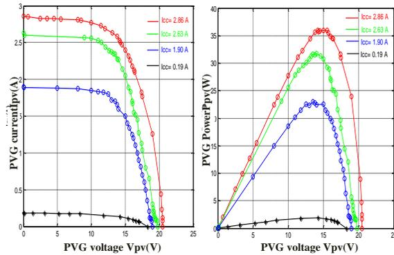
Fig. 7. External characteristic of photovoltaic panel for various illumination and temperature =  $26 C^\circ$ .
