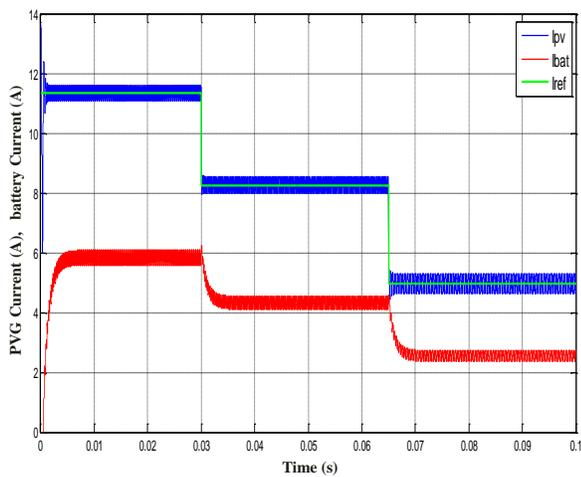
Fig. 17. Variation of the PVG and battery current for a constant temperature and variable illumination.
