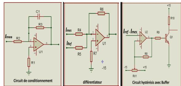
Fig. 20. Detailed diagram of the analogical loop of current.
