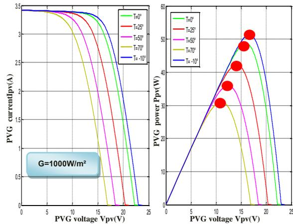
Fig. 5. PVG (current- voltage) and (power- voltage) characteristic for different temperatures.
