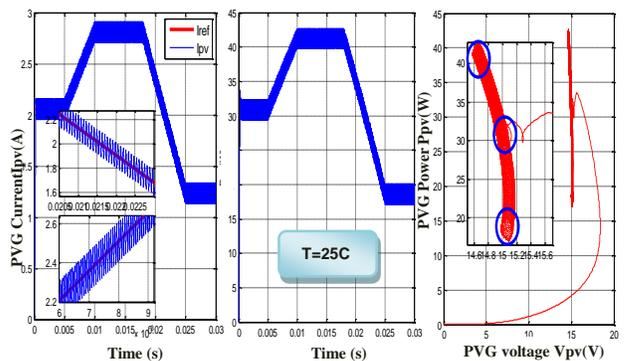
Fig. 15. Variation of the PVG power and current for a random illumination.
