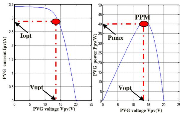
Fig. 3. PVG (current- voltage) and (power- voltage) characteristic for standards conditions.
