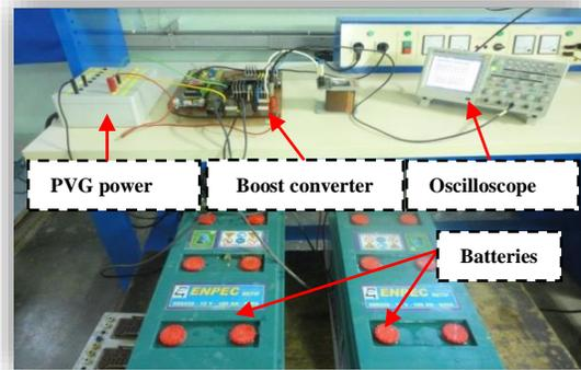
Fig. 19. Tests platform
