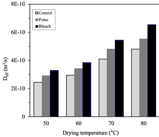
Figure 5. Effective moisture diffusivity versus temperature
