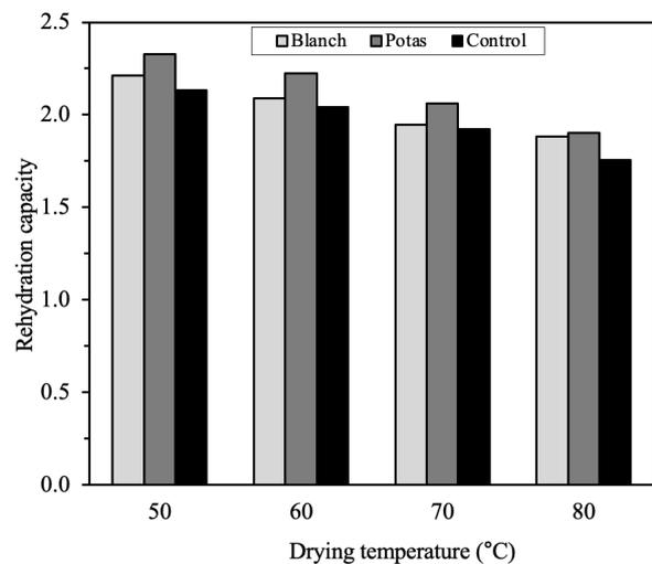
Figure 7. Effect of pre-treatment and air-drying temperature on rehydration capacity of peas
