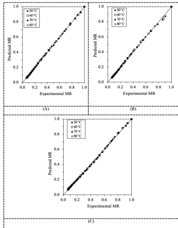
Figure 4. Comparison of experimental and predicted moisture ratio values using Page model (A: Potas, B: Blanch, C: Control)
