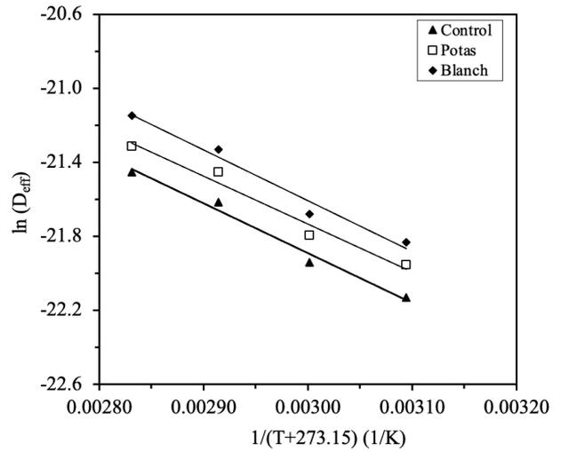
Figure 6. Arrhenius-type relationship between effective moisture diffusivity and temperature
