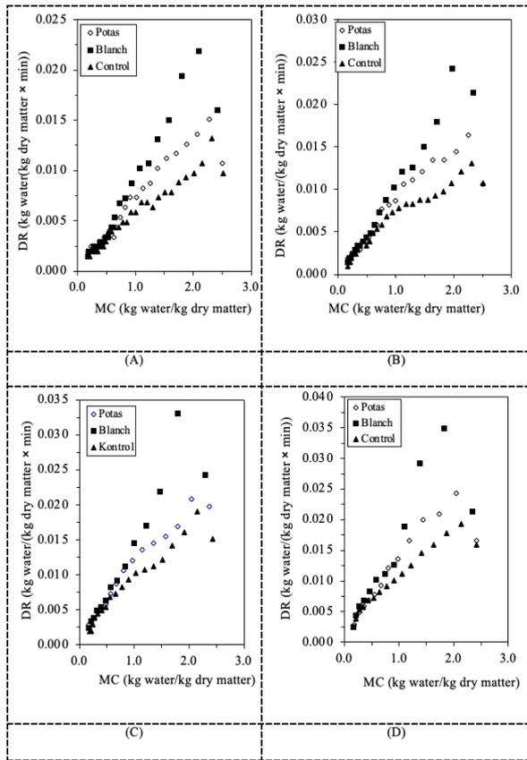
Figure 3. Moisture content vs drying rate for A: 50°C, B: 60°C, C: 70°C, D: 80°C
