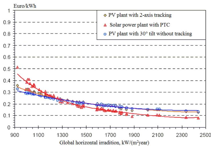
**Figure 2. Cost price of the generated power energy on solar power plants**
