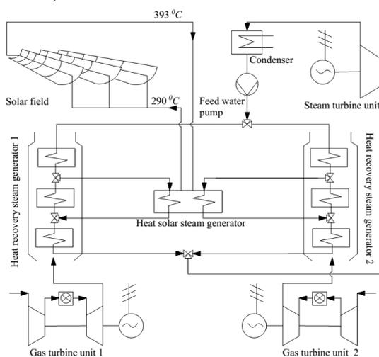
**Figure 4. ISCC system schematic diagram based on PTC**
