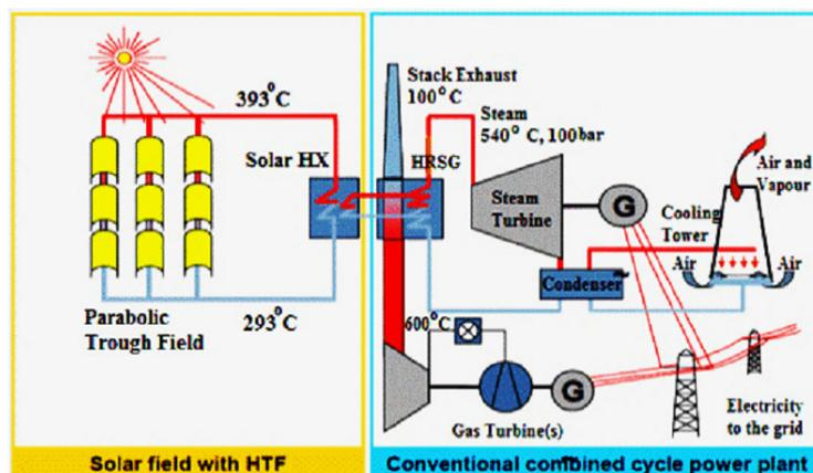
**Figure 1. ISCC system schematic diagram**
