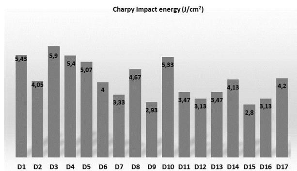
Figure 6. Notch impact analysis results for the samples.
