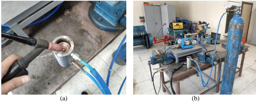
Figure 3. a) Copper casting mold, b) reverse vacuum casting system
