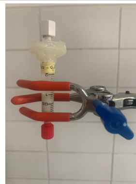
Figure 2. Experimental setup used to determine the breakthrough of Ge from column.
