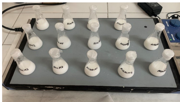
Figure 1. Experimental setup used to determine K_d under static conditions.
