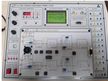
Figure 5: KL-75003 Electrooculogram (EOG) Module.
