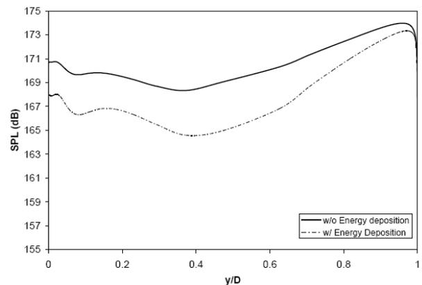
**Figure 9.** Pressure Distribution on Downstream Face of the Cavity before and after Energy Deposition
