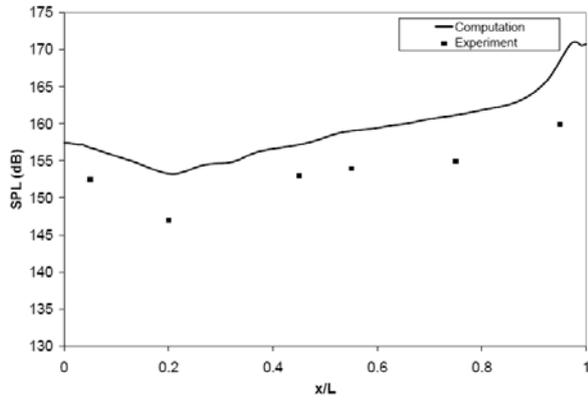
**Figure 4.** SPL Distribution on Cavity Floor (Without energy deposition)
