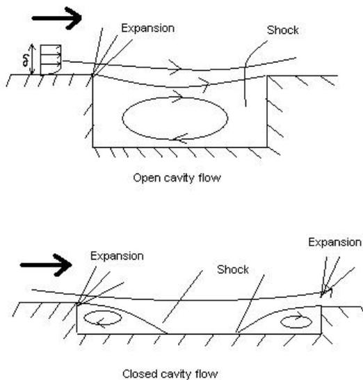
**Figure 1.** Types of Cavity Flows
