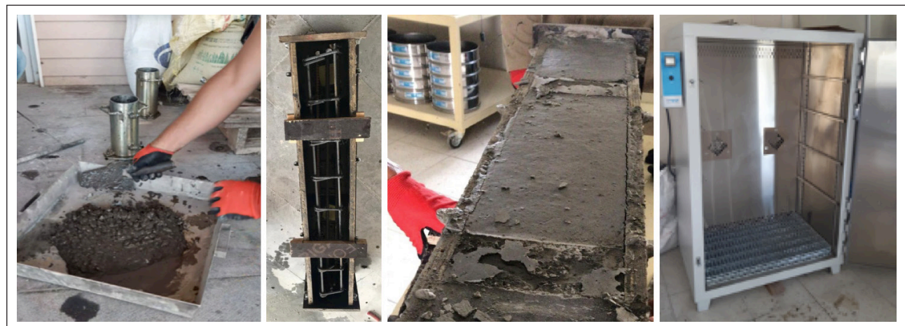
Figure 2. Placing and curing concrete in molds.
