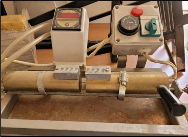
Figure 3. Thermal conductivity coefficient measuring device
