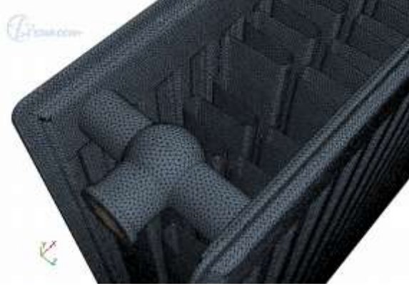
Figure 1. Mesh density of outer side of the panel radiator with TBOE connection
