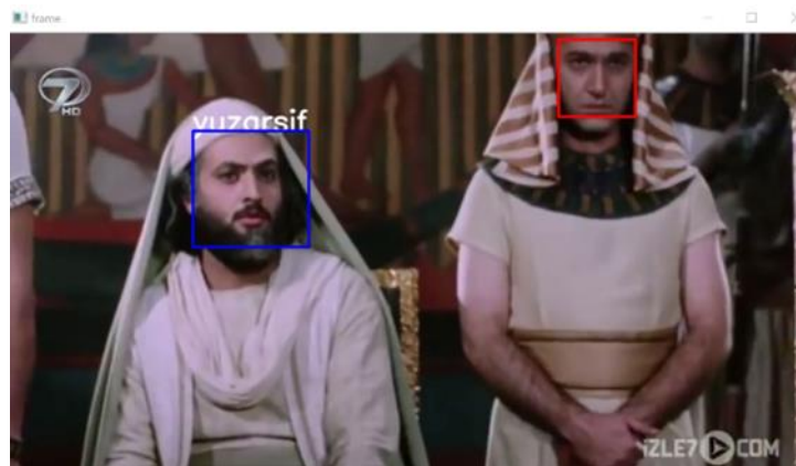
Fig. 6. The Recognized Face of The Person Who has been Trained in The project and The Unrecognized Face of A Random Person Who has not been Trained in The Project in Question [42].
