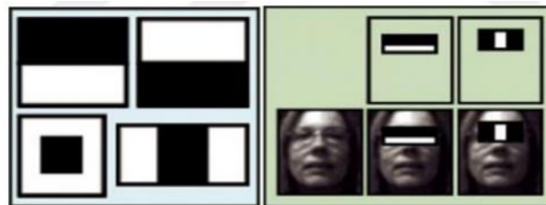
Fig. 3. Haar samples and Eye Detection [51]
