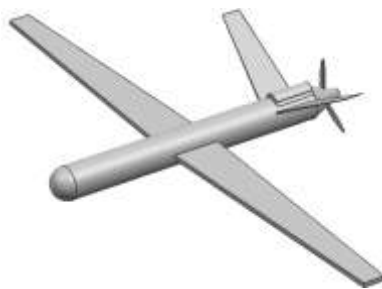
Figure 2a. A simplified geometry UAV, 3-dimensional view.
