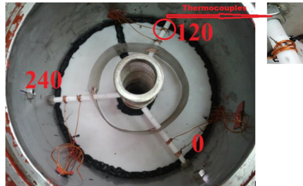
Figure 2. A top view of the adsorbent bed to show the location of the thermocouples
