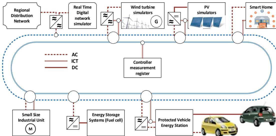
**Figure 1.** Main components of the smart grid system
