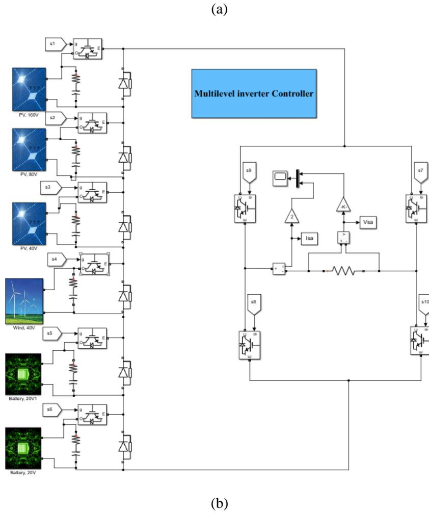
**Figure 1.** The proposed MLI with different RESs; (a) structure, and (b) model circuits.
