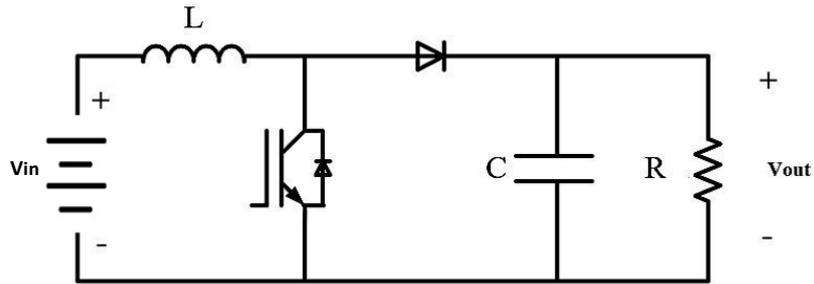
**Figure 2.** Circuit diagram of DC-DC step-up converter
