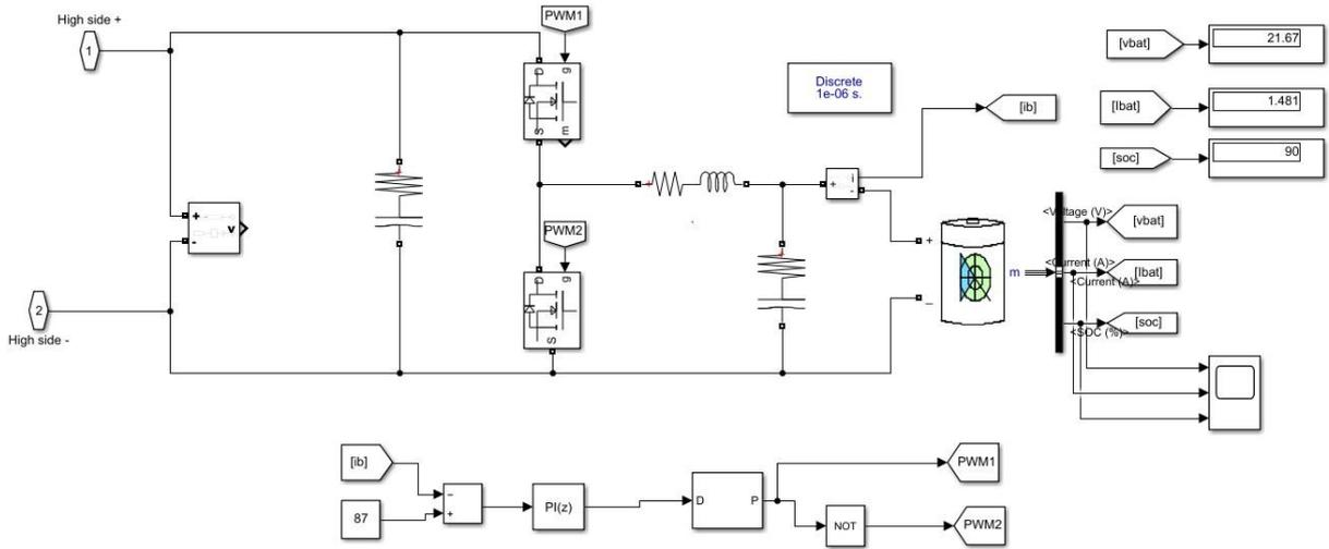
**Figure 6.** Battery circuit
