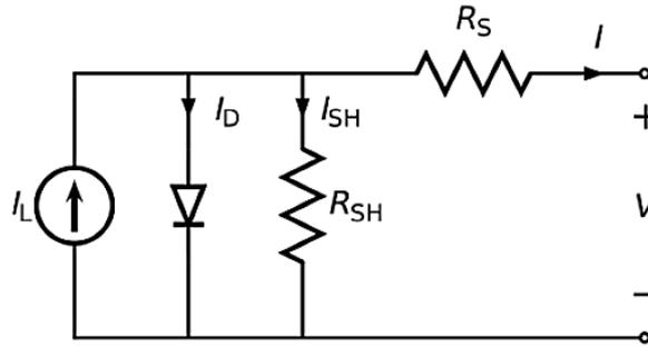
**Figure 3.** Circuit diagram of PV-cell
