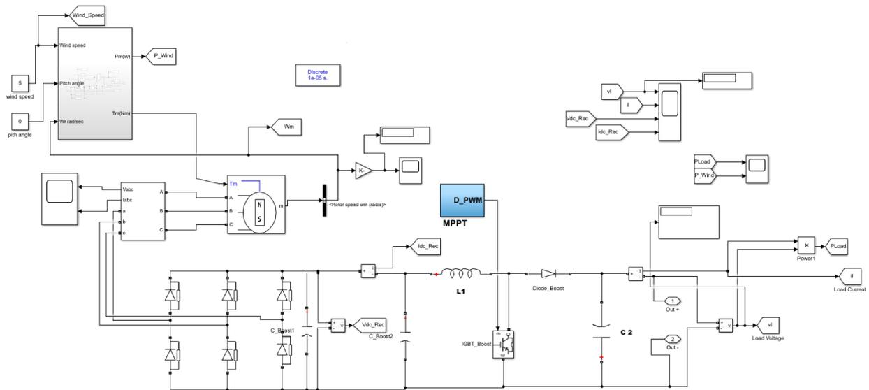
**Figure 5.** Wind Energy Conversion System based on PMSG
