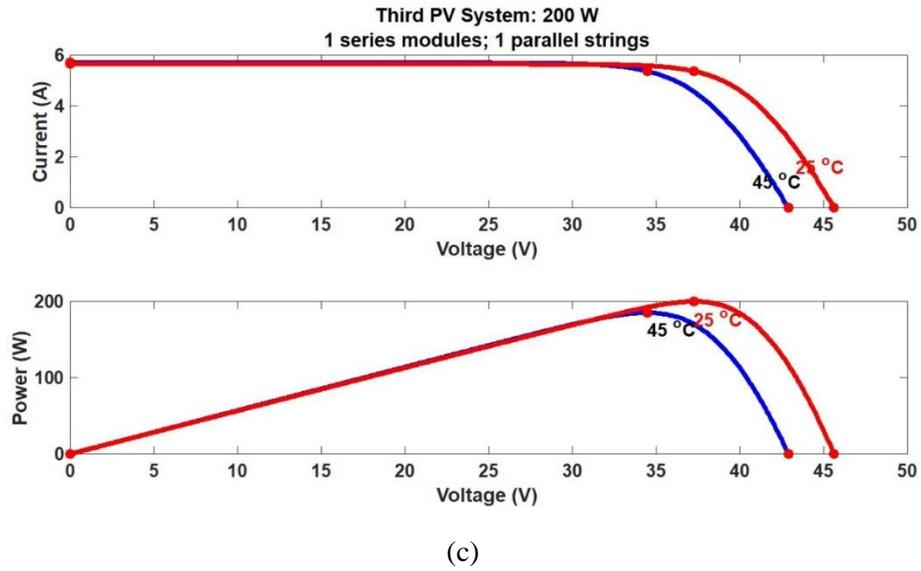
**Figure 4.** The (V-I) and (P-V) characteristics of (a) PV system 1 (b) PV system 2 (c) PV system 3
