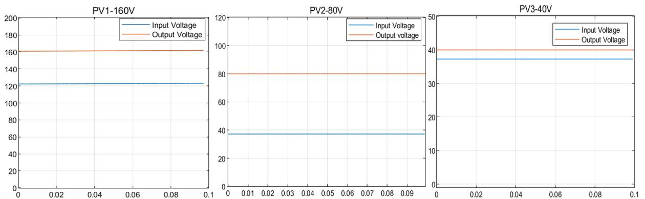
**Figure 7.** The input and output voltage of PV converter (a) PV system1 (b) PV system2, and (c) PV system3
