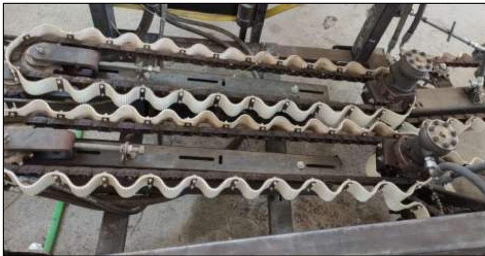
Figure 3. Product conveyor unit
