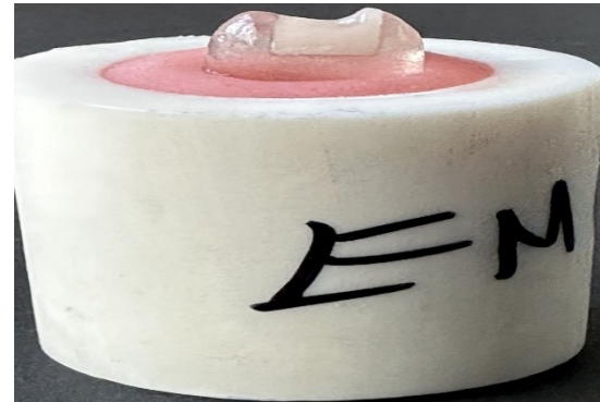
Figure 3: Sample embedded in acrylic resin
