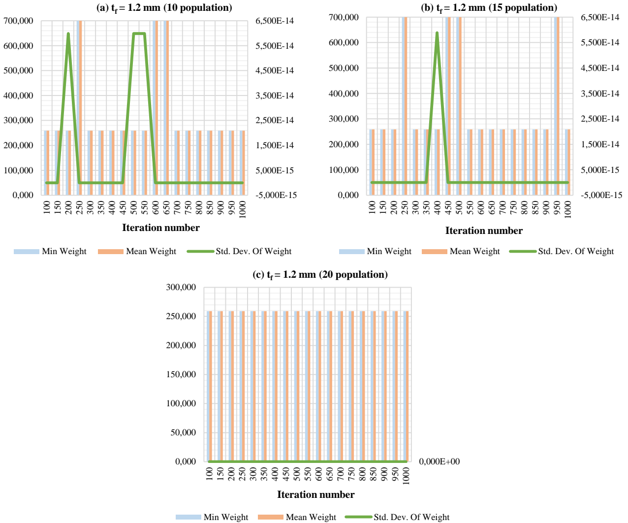
Figure 3. Distribution of min, mean and standard deviation of weight values according to iterations (PSO).
