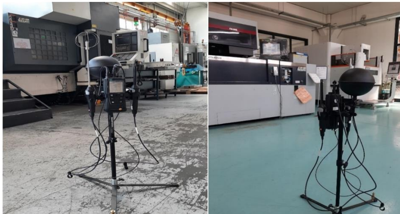
Figure 4: General view of Testo-480 at the time of measurement
