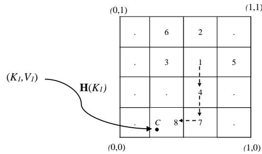
**Figure 1.** Partition of 2D coordinate space by the peers in CAN, mapping of a (key, value) pair and routing of a query  $(K_I)$  (from peer 1 to peer 8).
