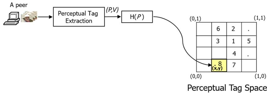
**Figure 2.** The proposed DHT based distributed perceptual tagging system as an analogue to the CAN design.
