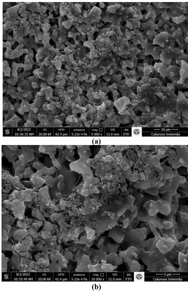
**Figure 6.** SEM image results of Ag-Ni-TiO<sub>2</sub>/Cordierite catalyst (a:5000x, b:10000x)
