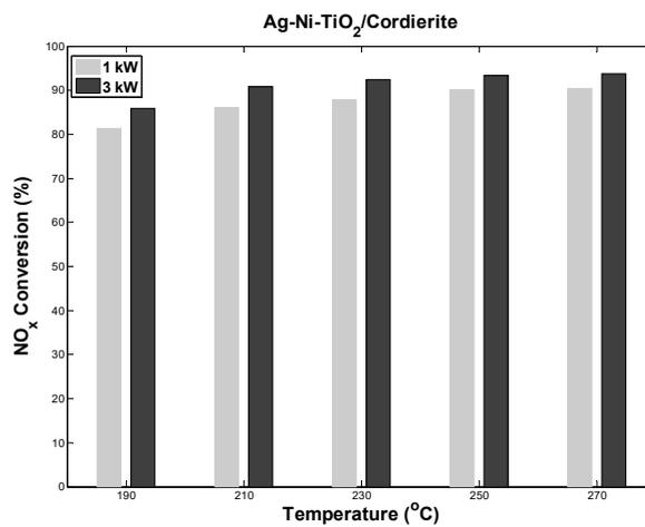
Figure 8. The NO<sub>x</sub> conversion results of the catalyst
