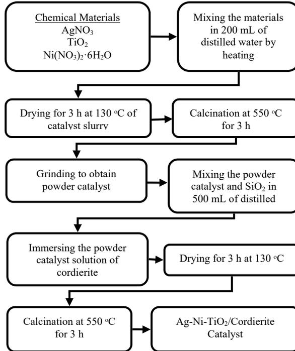
Figure 1. Steps in catalyst preparation
