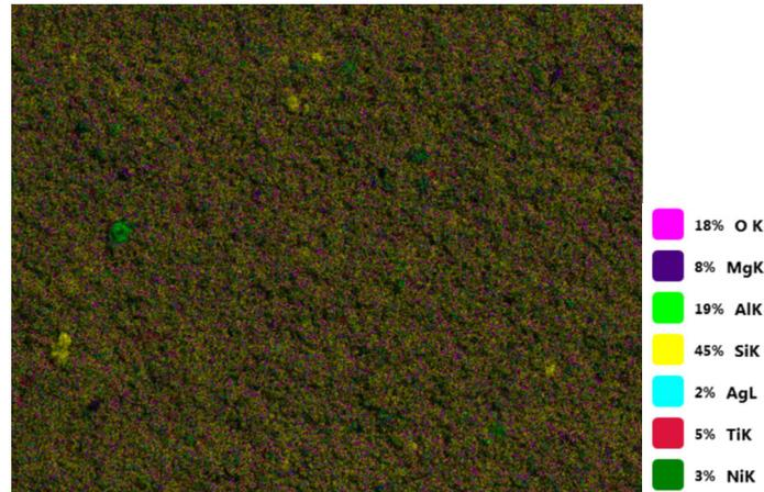
Figure 7. SEM mapping result of Ag-Ni-TiO<sub>2</sub>/Cordierite catalyst
