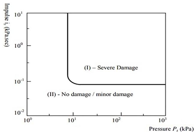
Figure 7: Typical pressure – impulse curve [8]
