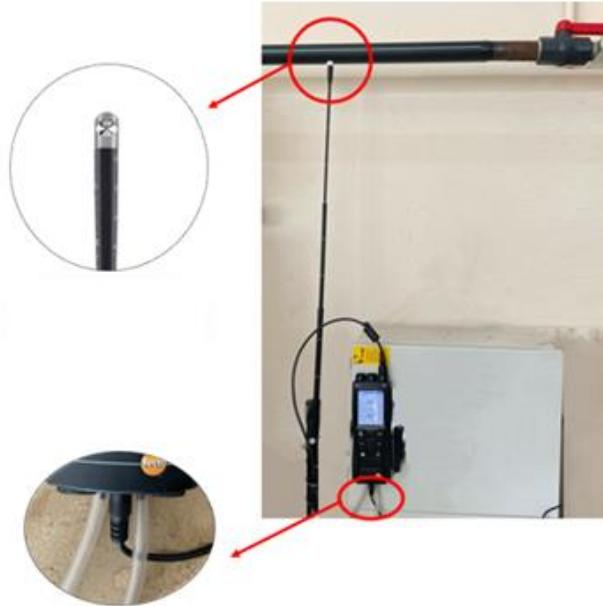
**Figure 2.** Digital air velocity and differential pressure meter.
