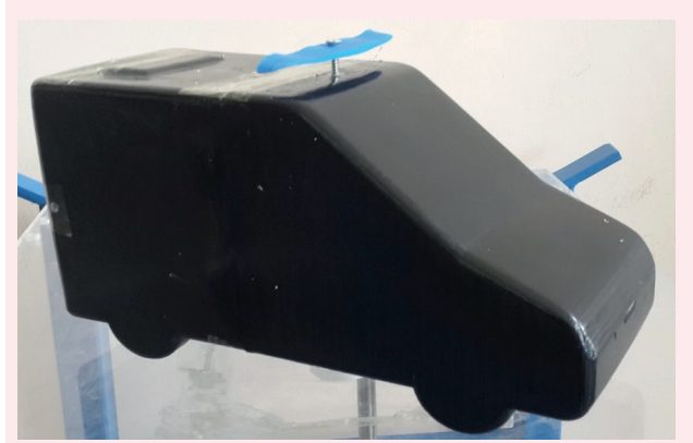
Figure 5. Test model 1 and front spoiler application
