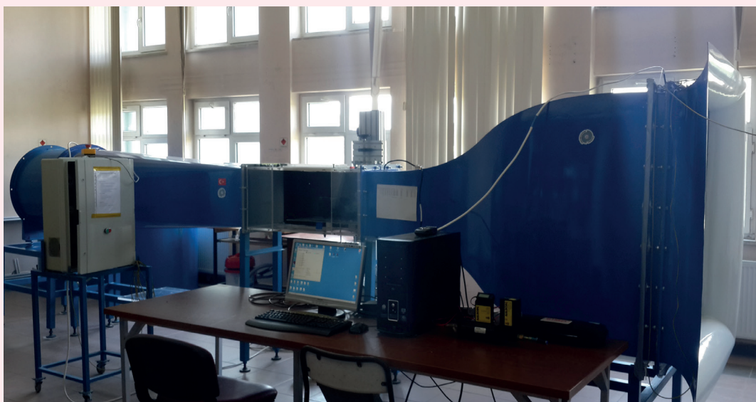
Figure 8. Suction-type wind tunnel and testing equipment
